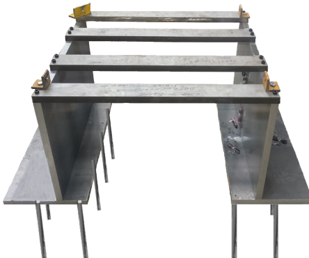
- Configuration 4. NO PU (Polyurethane) foam and NO piles connected
