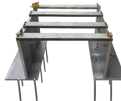
- Configuration 4. NO PU (Polyurethane) foam and NO piles connected
