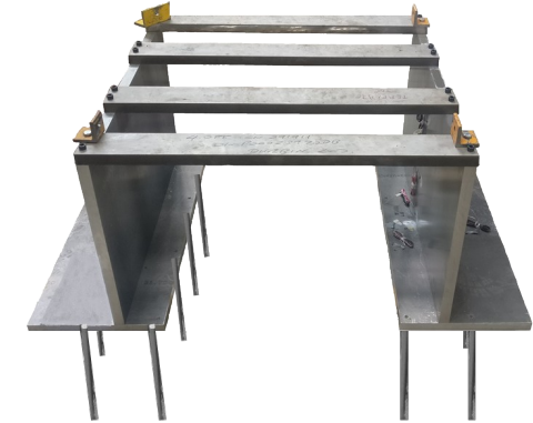
- Configuration 3. NO PU (Polyurethane) foam and piles connected
