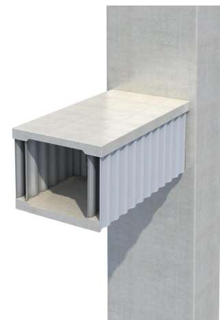
Figure 4 Corrugated Steel Web Steel-Concrete Composite Crossbeam
