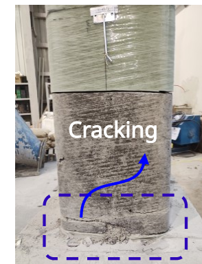
Failure modes of rubber concrete and steel tubes
