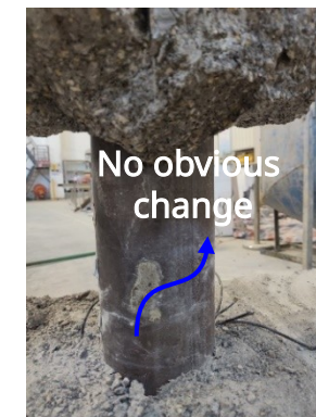
Failure modes of rubber concrete and steel tubes
