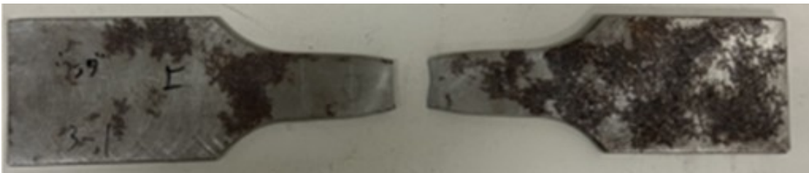
C3. Welding part of spiral pipe (Milled)
