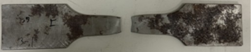
C3. Welding part of spiral pipe (Milled)
